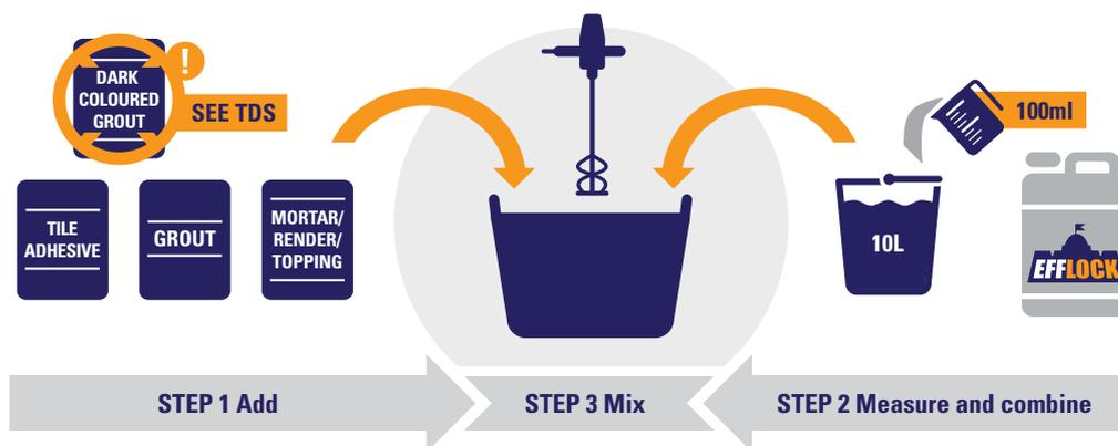
Efflock is a high performance, water based, VOC free, liquid additive designed for the bulk impregnation of cement based building materials to protect against efflorescence and damp.
